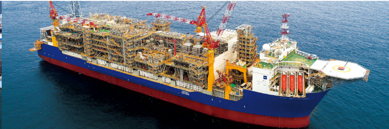
부유식 원유생산저장하역설비(FPSO, Floating Production, Storage, and Offloading)
